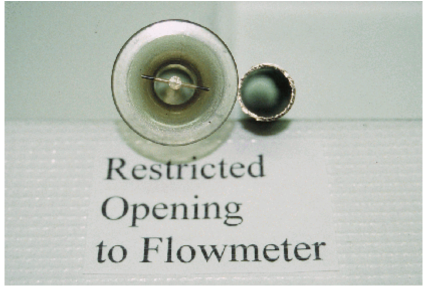
Figure C9 Restricted Opening – Flow Meter
